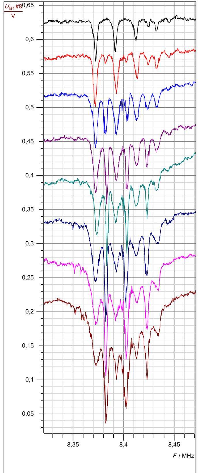
Fig. 6: Absorption spectrum for  $^{87}\text{Rb}$  with  $\sigma^+$  light at 0 dB attenuation and high-frequency amplitude increasing from top to bottom.
