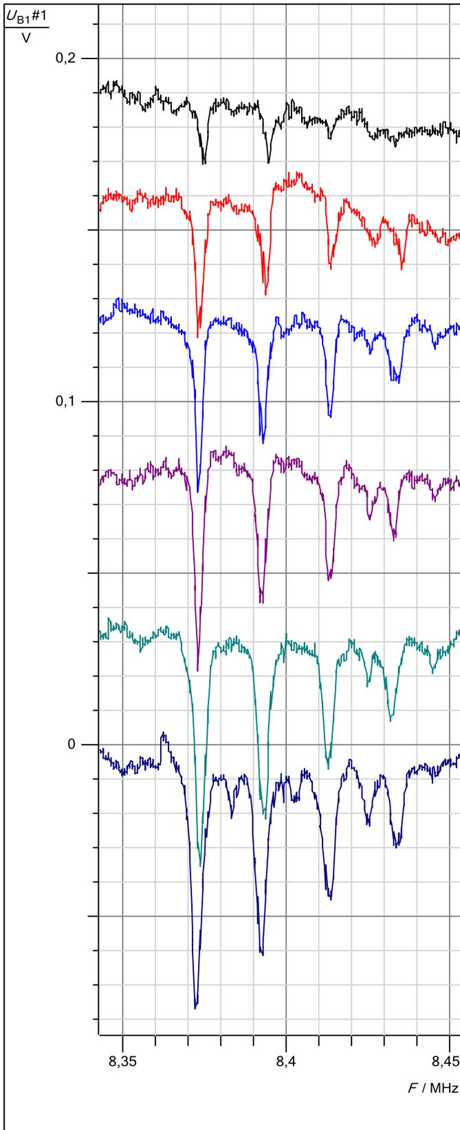
Fig. 5: Absorption spectrum for  $^{87}\text{Rb}$  with  $\sigma^+$  light at 20 dB attenuation and high-frequency amplitude increasing from top to bottom.
