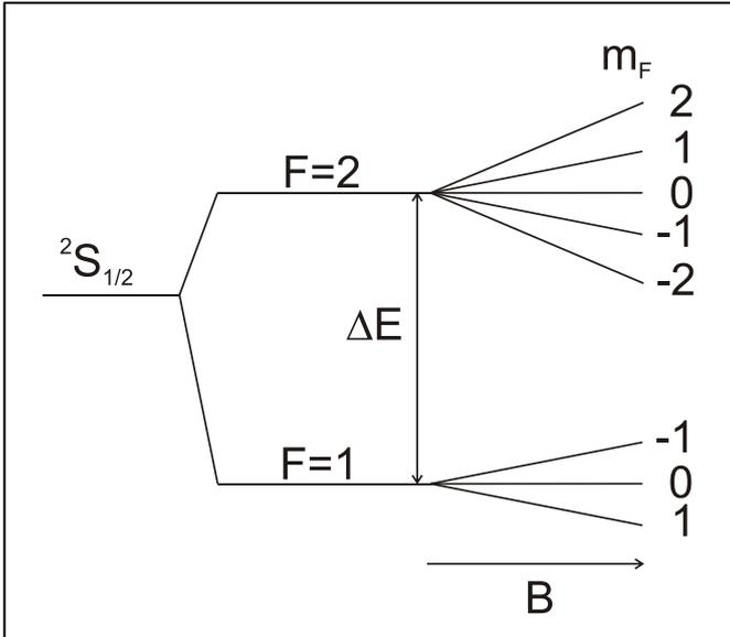
Fig. 1: Schematic representation of Zeeman levels in the ground state of  $^{87}\text{Rb}$  Hyperfine splitting  $\Delta E$  and Zeeman splitting are not drawn to scale.
