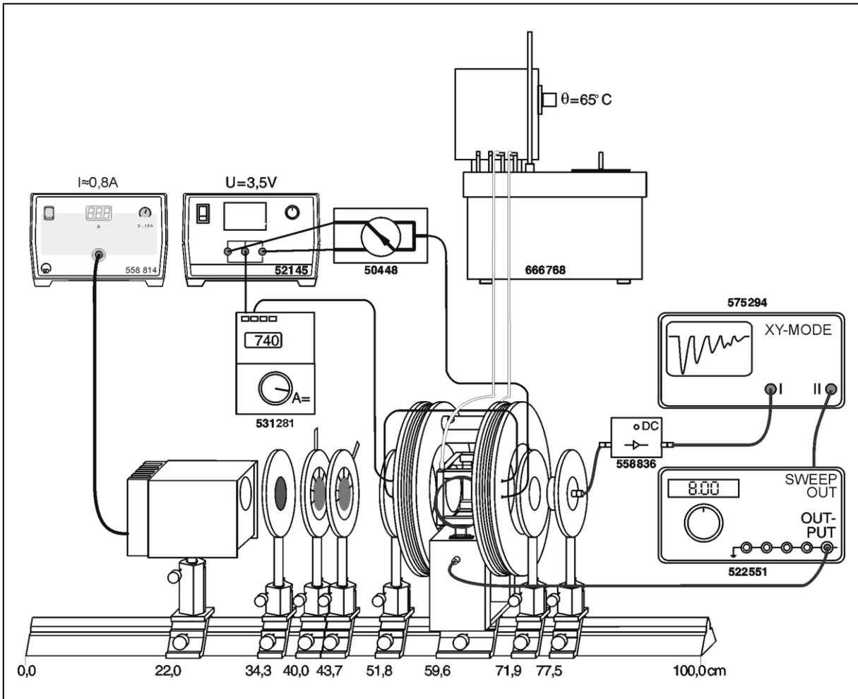
Fig. 2: Overview diagram of the entire experiment setup. Position specifications are measured from the left edge of the optical riders.
