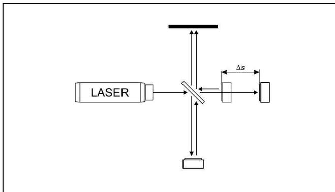
length of the affected beamlet. During this shift, the interference fringes move on the observation screen. The evaluation relies on counting either the maxima or the minima of intensity that pass by a defined point on the observation screen while shifting the plane mirror is.
