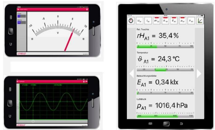
Fig. 4: Sensor-CASSY can also be sensibly used with smart phones and tablets.
