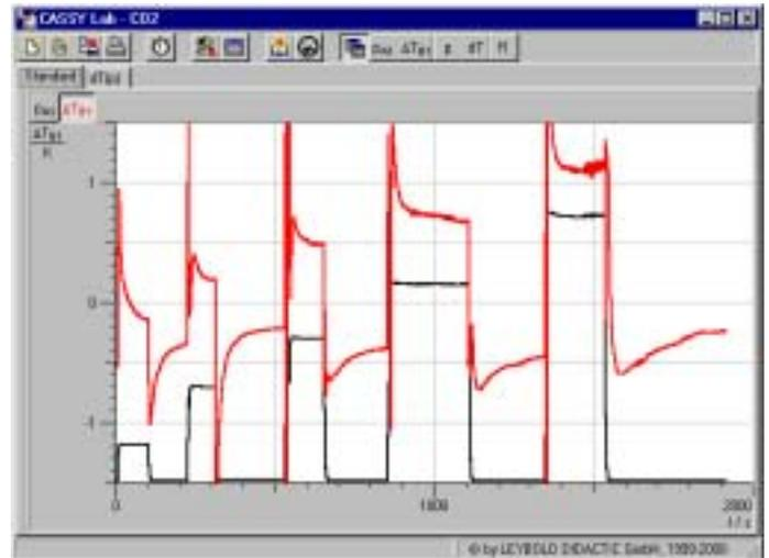
Pressure difference  $\Delta p$  and temperature difference  $\Delta T$  (as functions of time)
