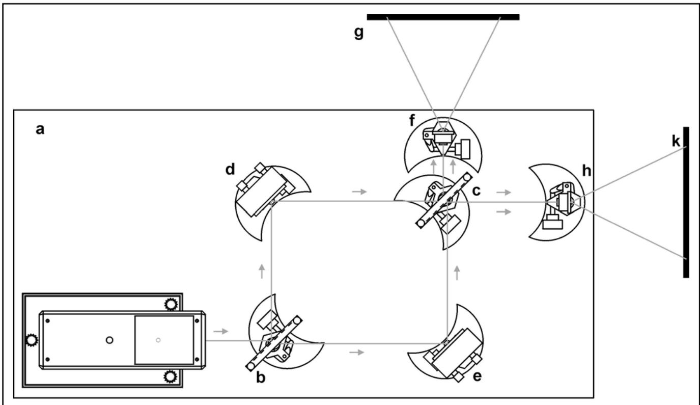
Illustration 1: Mach-Zehnder interferometer setup
