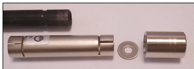
Fig. 6: Silver: Parts from 559 18 required to assemble the collimator, black: The radioactive preparation.
