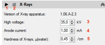
Fig. 3: X-ray setting: 1: X-ray on, 2: X-ray off, 3: High voltage, 4: Anode current, 5: X-ray hardness.
