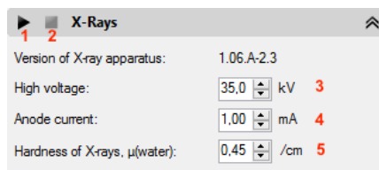
Fig. 3: X-ray setting: 1: X-ray on, 2: X-ray off, 3: High voltage, 4: Anode current, 5: X-ray hardness.
