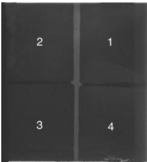
Fig. 5 Fogging of x-ray film at a constant product of  $I \cdot \Delta t$
