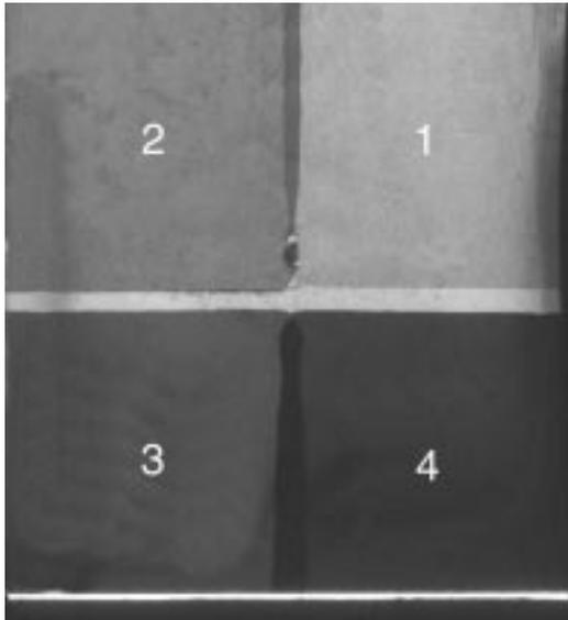
Fig. 4 Fogging intensities of the x-ray film at  $I = 1.00$  mA
