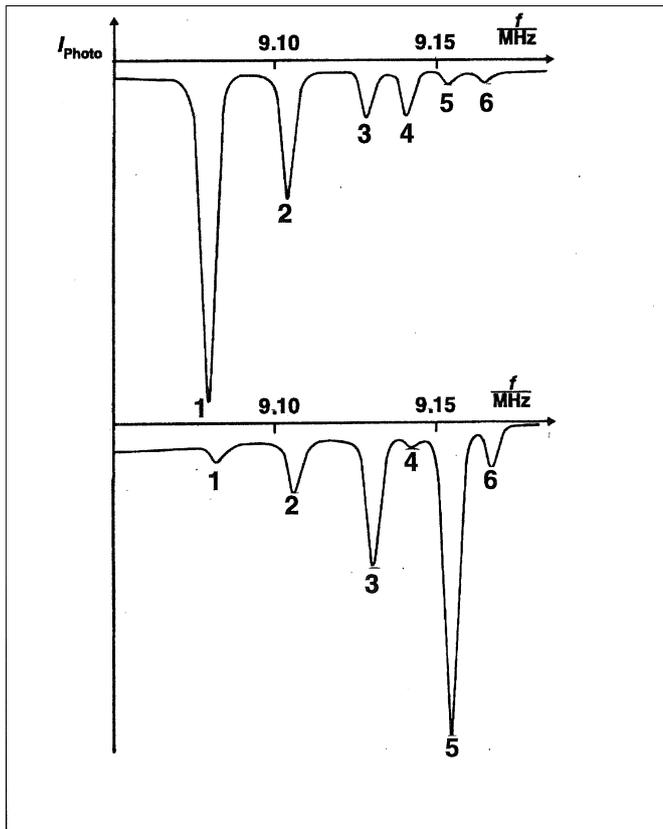
Fig. 5: Absorption spectrum  $^{87}\text{Rb}$  with  $\sigma^+$  light (top) and  $\sigma^-$  light (bottom). For identification of the absorption lines see Table 2.
