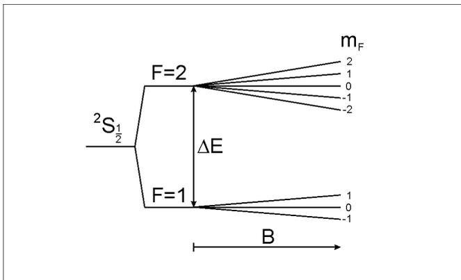
Fig. 2 Schematic representation of Zeeman levels in the ground state of <sup>87</sup>Rb. Hyperfine splitting  $\Delta E$  and Zeeman splitting are not drawn to scale.
