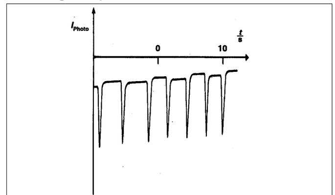
Fig. 5: Transmitted intensity as a function of time for multiple rapid reversals of the Zeeman magnetic field. The amplitude of the signal is a measure of the quality of the adjustment.
