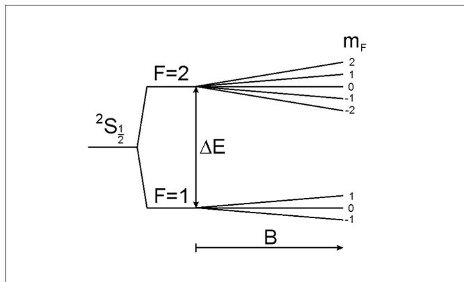
Fig. 2 Schematic representation of Zeeman levels in the ground state of  $^{87}\text{Rb}$  Hyperfine splitting  $\Delta E$  and Zeeman splitting are not drawn to scale.
