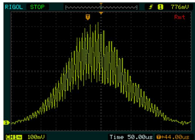
We see a strong scattering signal while the particle passes through the laser beams and there is a fast modulation due to the interference pattern.
