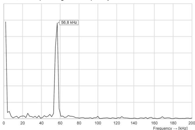
A modern oscilloscope is able to calculate the Fourier transform frequency spectrum of the measurement, usually by using a FFT. The result is shown above. The exact frequency is 56.8 kHz in this example.
