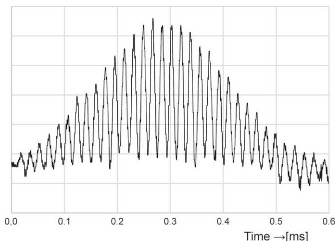
We can see that there are about 5.5 oscillations in a 100  $\mu$ s time, corresponding to a frequency of 55 kHz.
