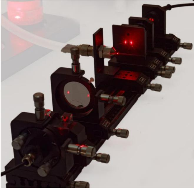
A particle moving through the interference fringes of two correctly crossing laserbeams will additionally show the high frequency modulation of the spatial interference pattern.
