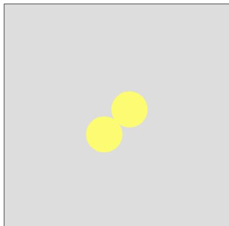
Fig. 3: Experimental result without polarizing filter on the translucent screen schematically. The image of the iris diaphragm due to the ordinary and extraordinary beam.
