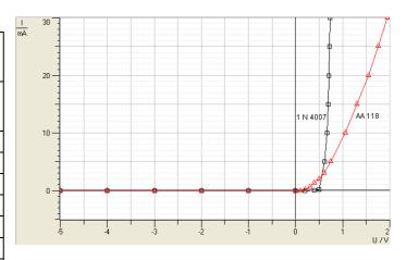
The current I of a diode in conducting state direction below the threshold voltage  $U_{\rm s}$  is close to zero increasing very fast above  $U_{\rm s}$ .
