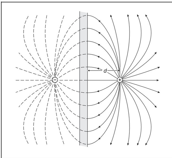
Fig. 1 The field lines of a pointlike charge  $Q$  in front of a metal plate in comparison with the field lines of two charges  $Q$  and  $-Q$ .
