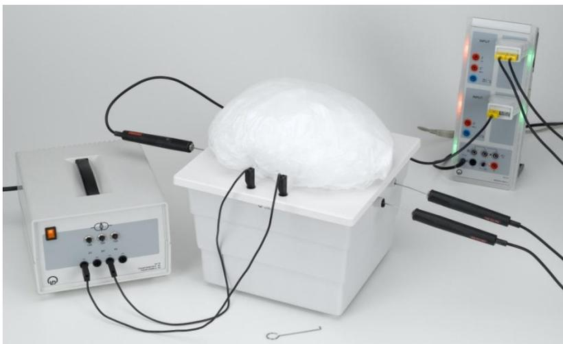
Fig. 1: Experiment setup: Determination of the thermal conductivity using the heat flux plate principle.
