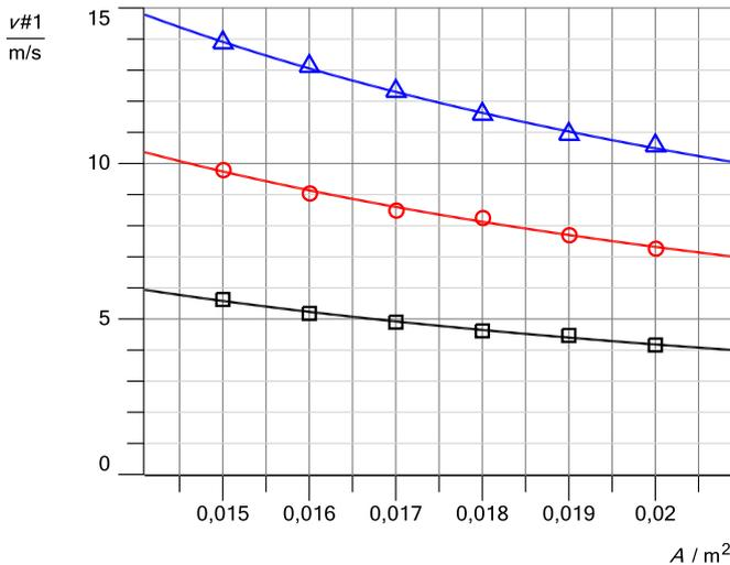
Fig. 7: Flow velocity  $v$  as a function of cross-sectional area  $A$  for three different wind speeds of the fan. The solid curve corresponds to a fit of a  $1/A$  hyperbola.
