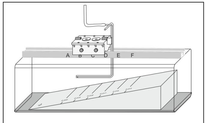
Fig. 8: Experimental setup for measuring the total pressure  $p_{\text{tot}}$ .
