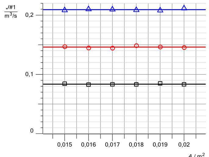
Fig. 5: Volume flow  $J$  as a function of the cross-sectional area  $A$  for three different wind speeds of the fan. The solid lines indicate the average value of one series of measurement.
