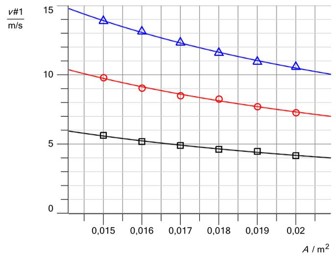
Fig. 6: Flow velocity  $v$  as a function of cross-sectional area  $A$  for three different wind speeds of the fan. The solid curves correspond to a fit of  $1/A$  hyperbolas.
