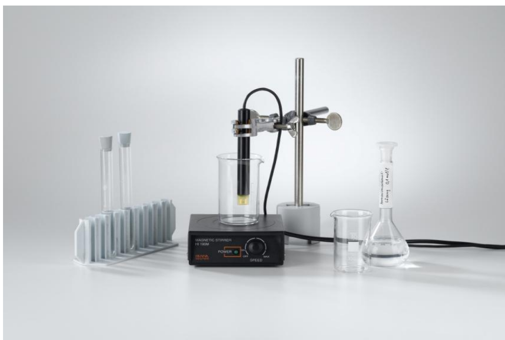
Fig. 1: Set-up of the experiment for conductivity measurement.
