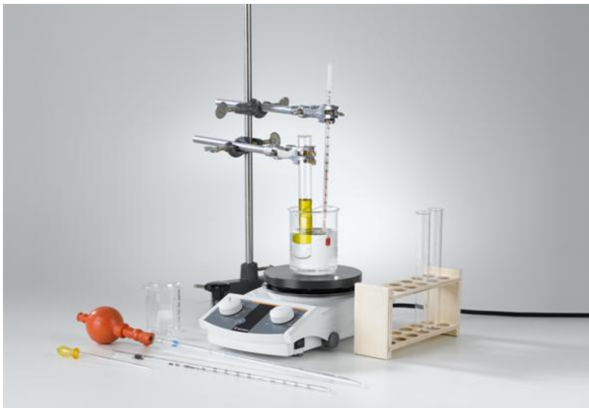
Fig. 1: Set-up of the experiment for the production of fuel from rapeseed oil.
