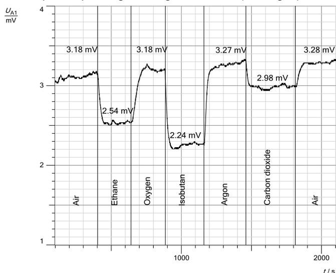
Fig. 2: Example measurements of various gases.
