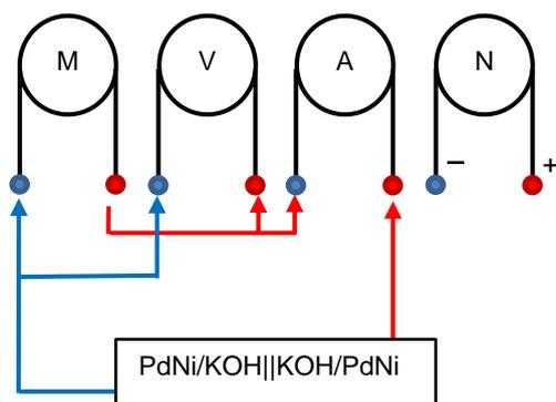
Fig. 4: Circuit of the experiment during power draw at the fuel cell.
