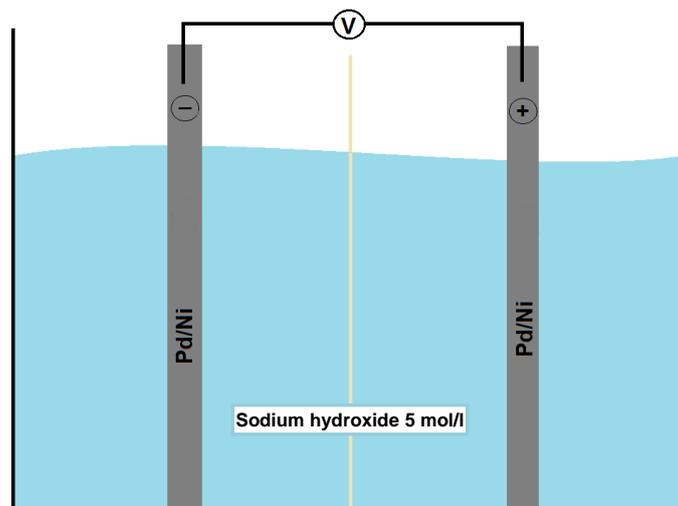
Fig. 2: Sketch of the experiment. Extraction of power from the fuel cell previously generated.
