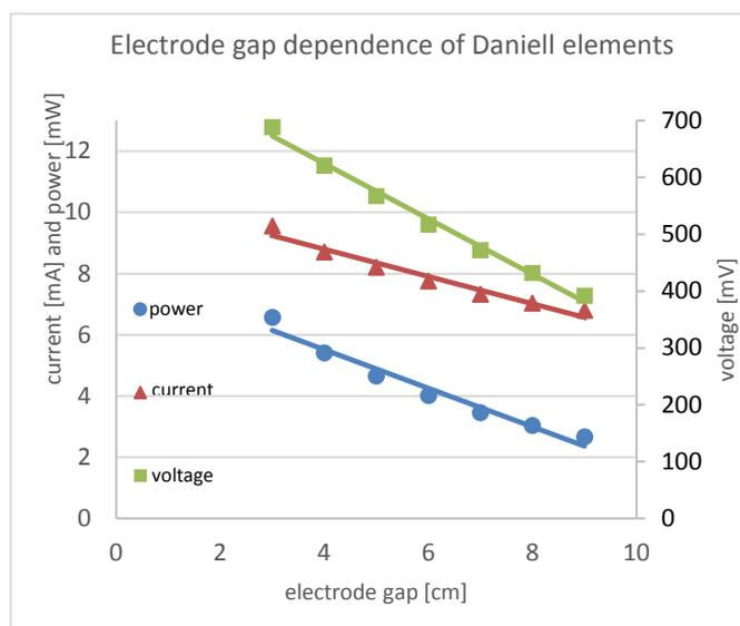
**Fig. 5:** Graphical evaluation of the gap measurements.
