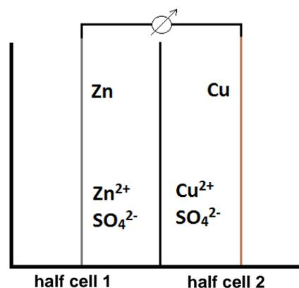
Fig. 2: Schematic of a Daniell cell
