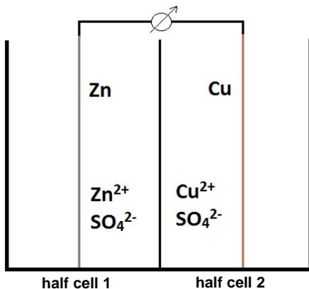
**Fig. 1:** Schematic of a Daniell cell. Both half cells must be separated by a paper diaphragm so that the solutions do not mix.
