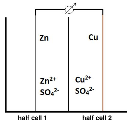
Fig. 2: Schematic of a Daniell cell
