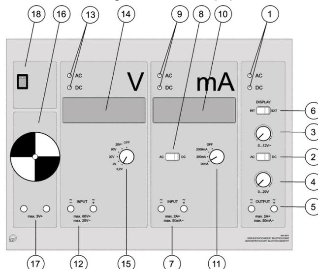
Fig. 3: Sketch of the demonstration unit.
