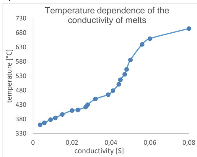
**Fig. 4:** Graphical plotting of temperature against conductivity.
