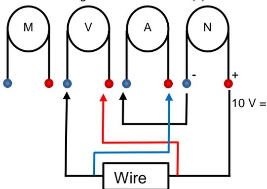
Fig. 3: Demonstration unit circuit for decoupling the internal resistance.
