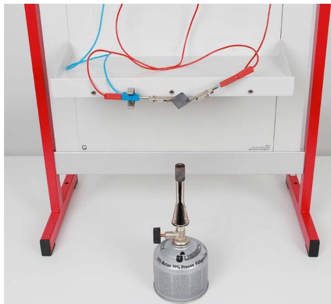
Fig. 4: Arrangement for stable fastening of the silicon disc.
