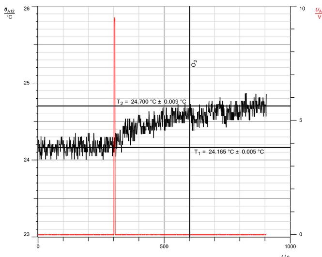
**Fig. 3:** Temperature and voltage measurements during the combustion of benzoic acid.
