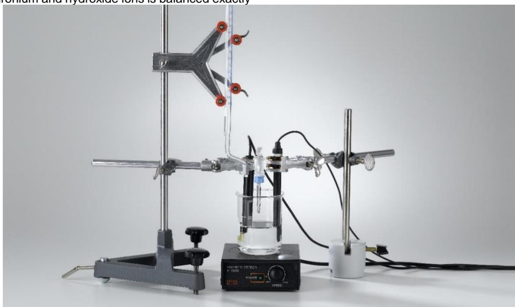
Fig. 1: Experiment apparatus for a conductometric titration with pH measurement.
