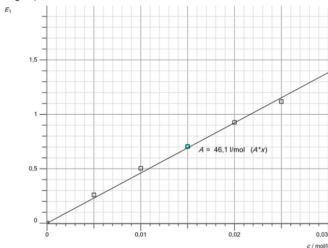
**Fig. 2:** Plotting the absorbance in dependence on the concentration of the tetraminecopper solution. The slope of the straight line is  $A = 46.1 \text{ L/mmol}$ .
