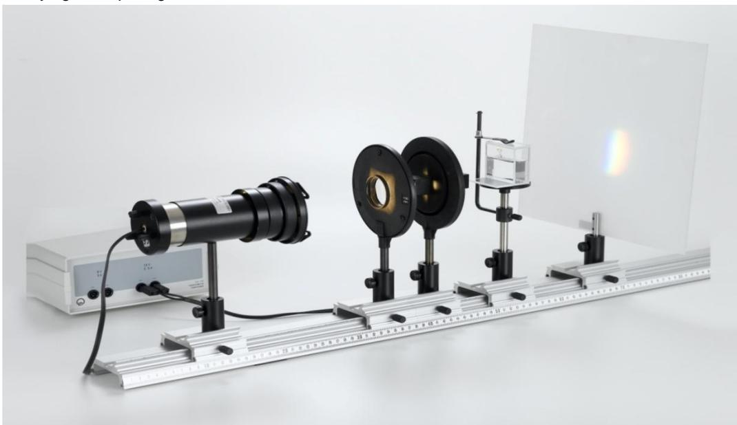
Fig. 1: Experimental apparatus for displaying the absorption spectra of dyes on a screen.
