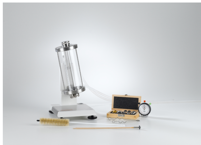
Fig. 1: Falling ball viscometer according to Höppler.
