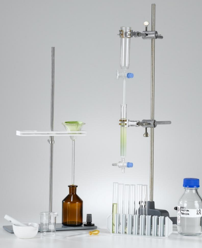
Fig. 1: Set-up of the experiment. Left: Production of the leaf extract. Right: Column chromatography.
