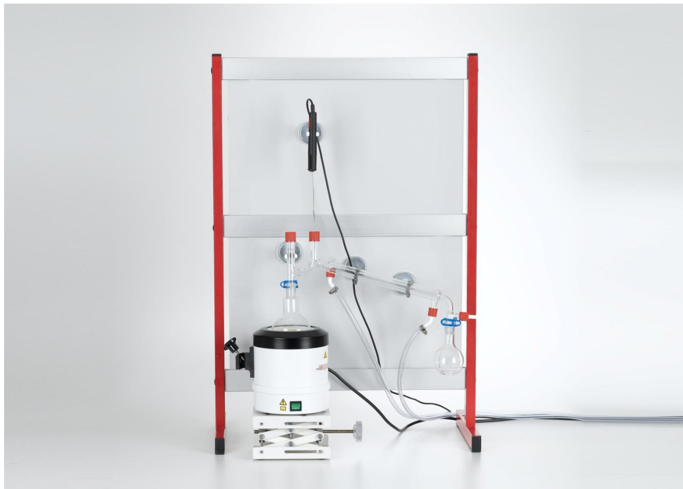
Fig. 1: Experimental apparatus for the distillation of red wine.
