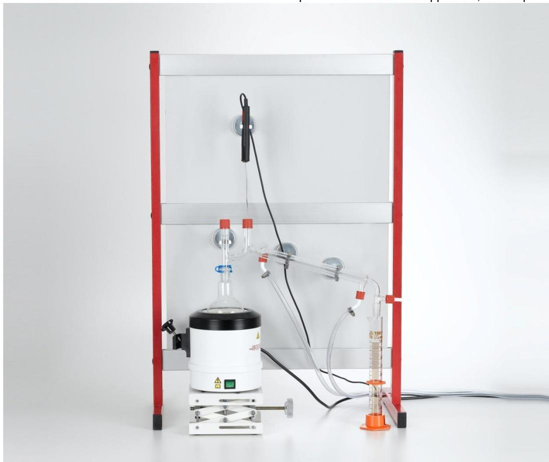
Fig. 1: Experimental apparatus for determining the boiling point of petroleum ether.
