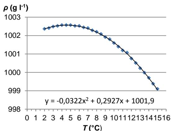
**Fig. 3:** Determining the density maximum. To do this, the density calculated from the vertical height is plotted against the temperature. The formula of the polynomial trend line is indicated.
