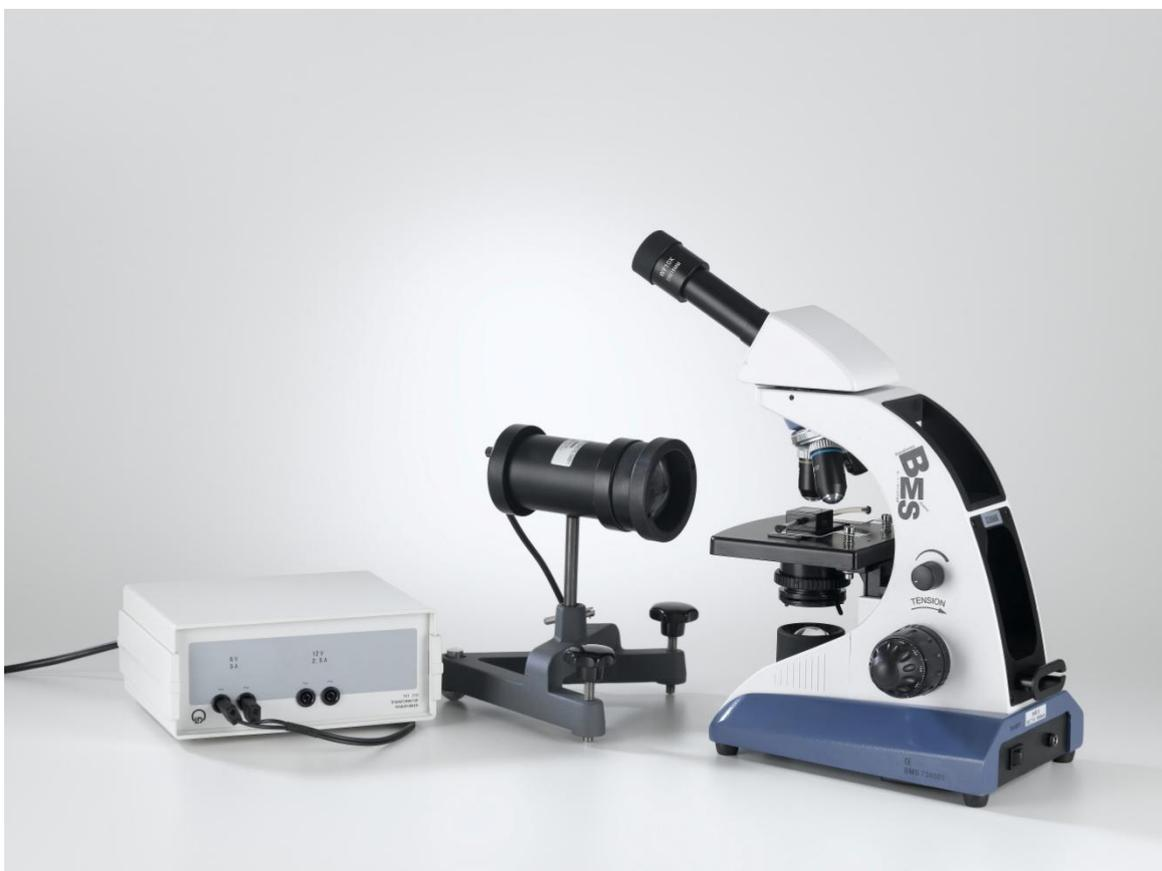
Fig. 1: Set-up for observing Brownian motion of smoke particles in air.
