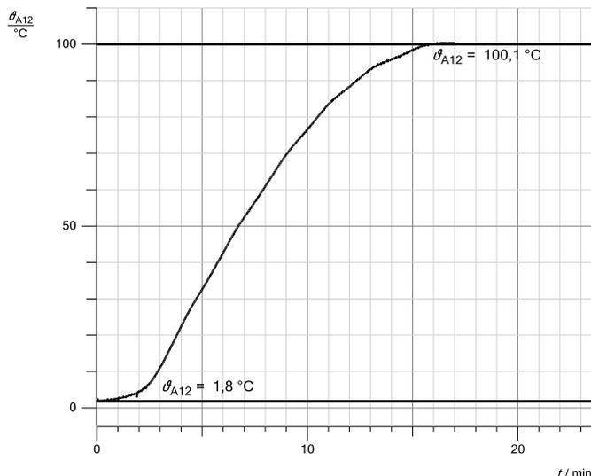
Fig. 2: Melting and boiling diagram for water.
