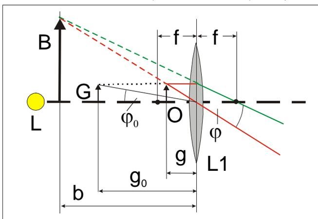
The first case concerns the observation of small objects when even the reduction of the object distance  $g$  to a minimum distance of  $g_0 = 25$  cm (i.e. the clear field vision) does not result in a small angle of vision. The latter case of a large object distance  $g$  is described in experiment P5.1.4.2.
