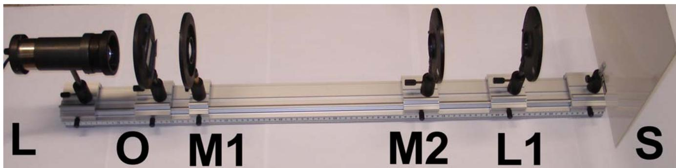
Fig. 9: Schematic representation of the experimental setup of the **microscope**. L: lamp, O: holder with object, M1: objective, M2: ocular (or eyepiece), model of eye consisting of L1: lens of the eye and S: translucent screen (retina of the eye).
