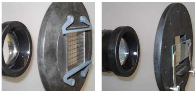
Fig. 3: How to use the holder with spring clips with various objects: (left) with grid object (taken from the pair of objects 461 66), (right) with glass scale (311 09).
