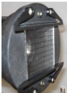
Fig. 4: How to setup the object directly at the aspherical condenser (460 20). For the resulting image on translucent screen (i.e. retina of the eye) see Fig. 6 left.
