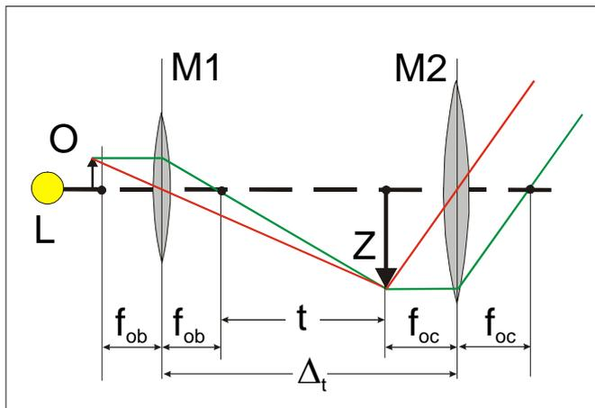
Fig. 2: Schematic representation of the microscope. M1: objective, M2: ocular, L: lamp, O: (small) object, Z: intermediate image, t: tube length,  $\Delta_t$ : distance between objective and ocular,  $f_{ob}$ : focal length of objective,  $f_{oc}$ : focal length of ocular
