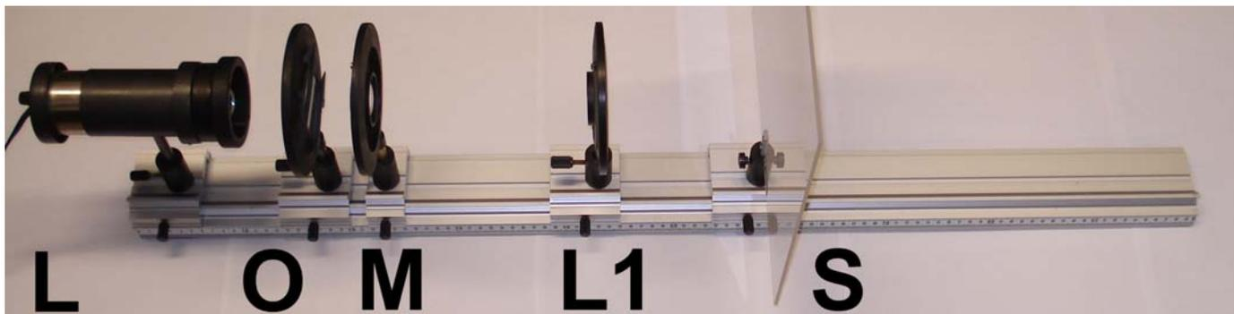
Fig. 7: Schematic representation of the experimental setup for the model of the **magnifier**. L: lamp, O: holder with object, M: magnifier (i.e. collecting lens) and model of eye, i.e.: L1: lens (of the eye), S: translucent screen (retina of the eye).
